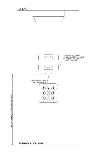
It is stated that pendants should be clear 2000mm from floor to bottom of pendant e.g. 3mtr floor to ceiling height = 1mtr long pendant
